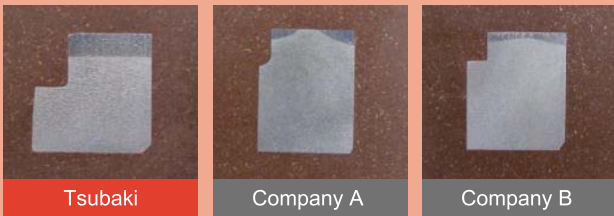
Cross-section observation of tooth hardened layer depth (darker area is the hardened layer)
