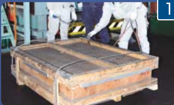
Chain is packaged in a special wooden box and delivered horizontally.
