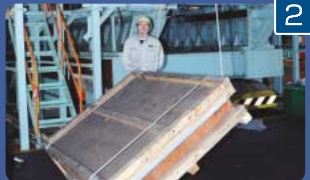
Stand wooden box upright when removing chain. (Be careful when standing wooden box.)
